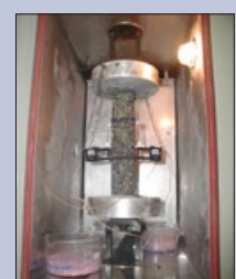
Thermal Stress Restrained Specimen Test (©BRRC)
