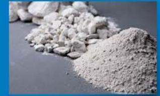
Lime is a product derived from limestone in an industrial process. Naturally occurring limestone, which is composed almost exclusively of **calcium carbonate** [ $\text{CaCO}_3$ ], transforms into quicklime [**calcium oxide** ( $\text{CaO}$ )] by heating. When slaked with water, quicklime transforms into hydrated lime, which is a dry powder composed of **calcium hydroxide** [ $\text{Ca}(\text{OH})_2$ ].
