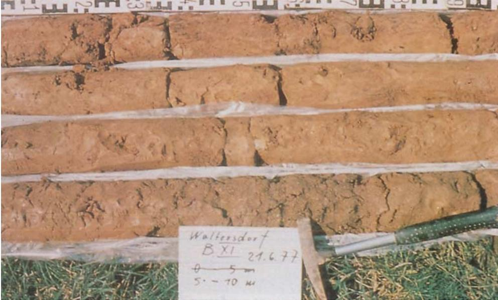
Figure 1. Ground investigation bore 1977 – soft silts in the hollow.
