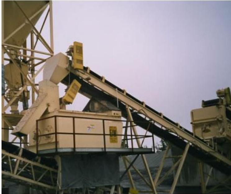
Figure 2: Pugmill used to mix hydrated lime with the wet aggregate in South Carolina (from [11]).
