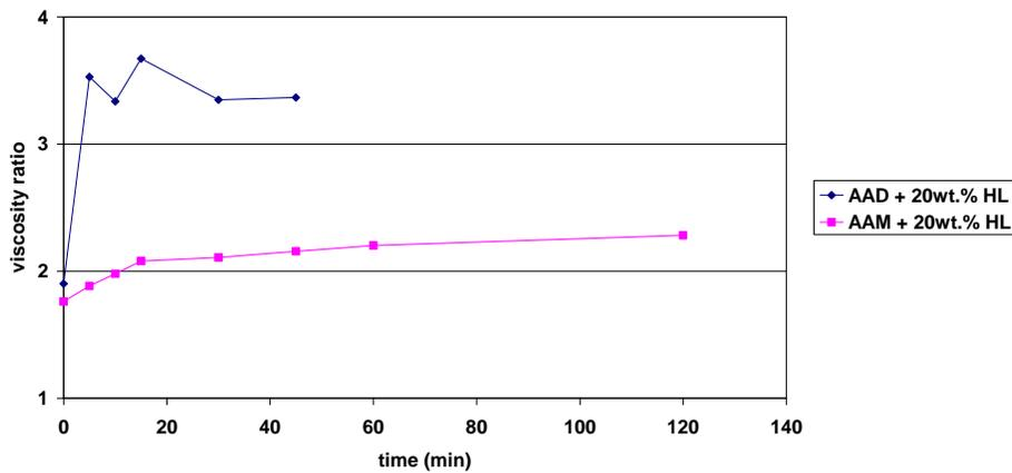
**Figure 7: Kinetics of viscosity build-up at 138°C for two bitumens modified with 20% hydrated lime. The viscosity stabilizes quickly for AAD when it keeps increasing after 120min for AAM. The neat bitumen did not show any significant viscosity change in the mean time (after [41]).**
