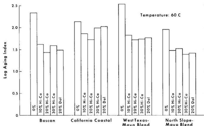
**Figure 4: Aging index at 60°C (viscosity after ageing divided by the viscosity before) for various sources of bitumen modified with different weight proportions of hydrated lime (Hi-Ca) and hydrated dolomitic lime (Dol). Ageing was performed in the Thin Film Accelerated Aging Test (TFAAT) corresponding to 3 days at 113°C under air exchange (from [33]).**
