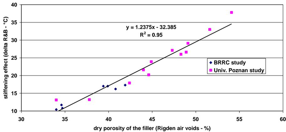
**Figure 6: Correlation between the stiffening effect of several fillers with their dry porosity (Rigden air voids). The data are from two studies: one from the Belgian Road Research Center [17] and the other from Poznan University [18].**
