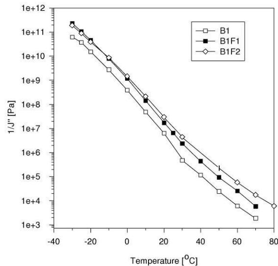
**Figure 8: Temperature dependence of the stiffening effect of hydrated lime as compared to limestone filler: inverse of the imaginary compliance ( $1/J''$ ) at 10 rad/s versus temperature for a 70/100 bitumen (B1) and the same bitumen with 50wt.% of limestone filler (B1F1) or mixed limestone filler containing 40% hydrated lime (from [46]).**
