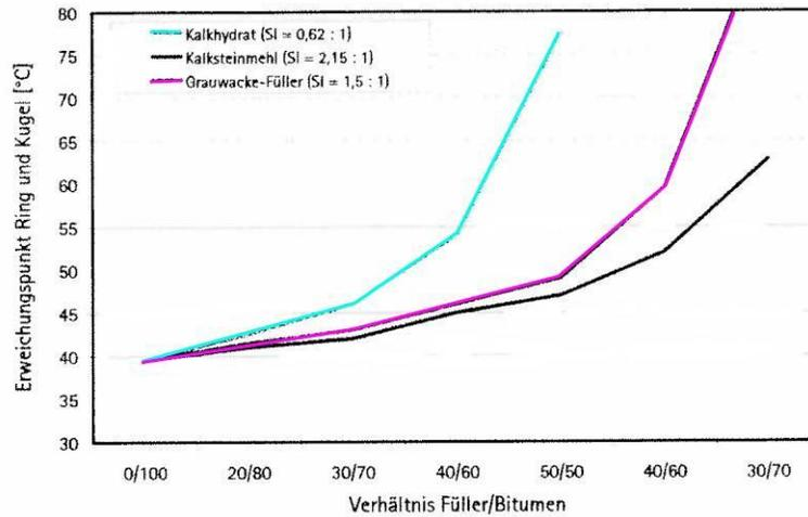
**Figure 1: Ring and ball softening temperature of a 200 penetration grade bitumen as a function of filler weight content (expressed in filler/bitumen wt.%/wt.%) for hydrated lime (Kalkhydrat), limestone filler (Kalksteinmehl) and Grauwacke filler (from [19]).**
