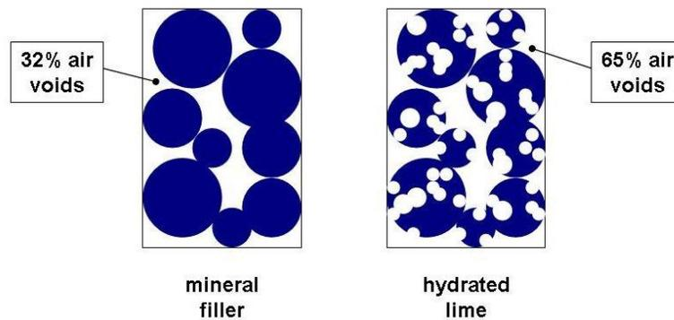
**Figure 5: The dry porosity of hydrated lime (right) is higher than that of mineral filler (left) because the porosity inside the particles, which is negligible with mineral filler, sums up to the porosity between particles.**
