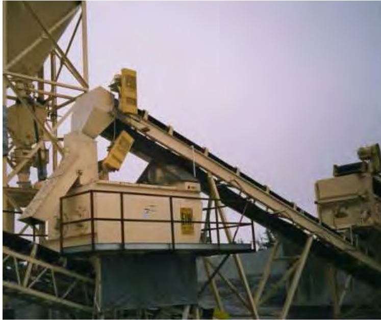
Figure 29: Pugmill used to mix hydrated lime with the wet aggregate in South Carolina (from [145]).
